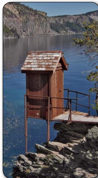
What resembles an outhouse at the bottom of the Cleetwood Cove Trail is actually a scientific instrument. Installed by the US Geological Survey in 1961—and now solar-powered—it measures the lake level, with great precision, every half hour. You can view (and graph) the data online.
